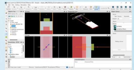
Structures for OVL Error Simulation
